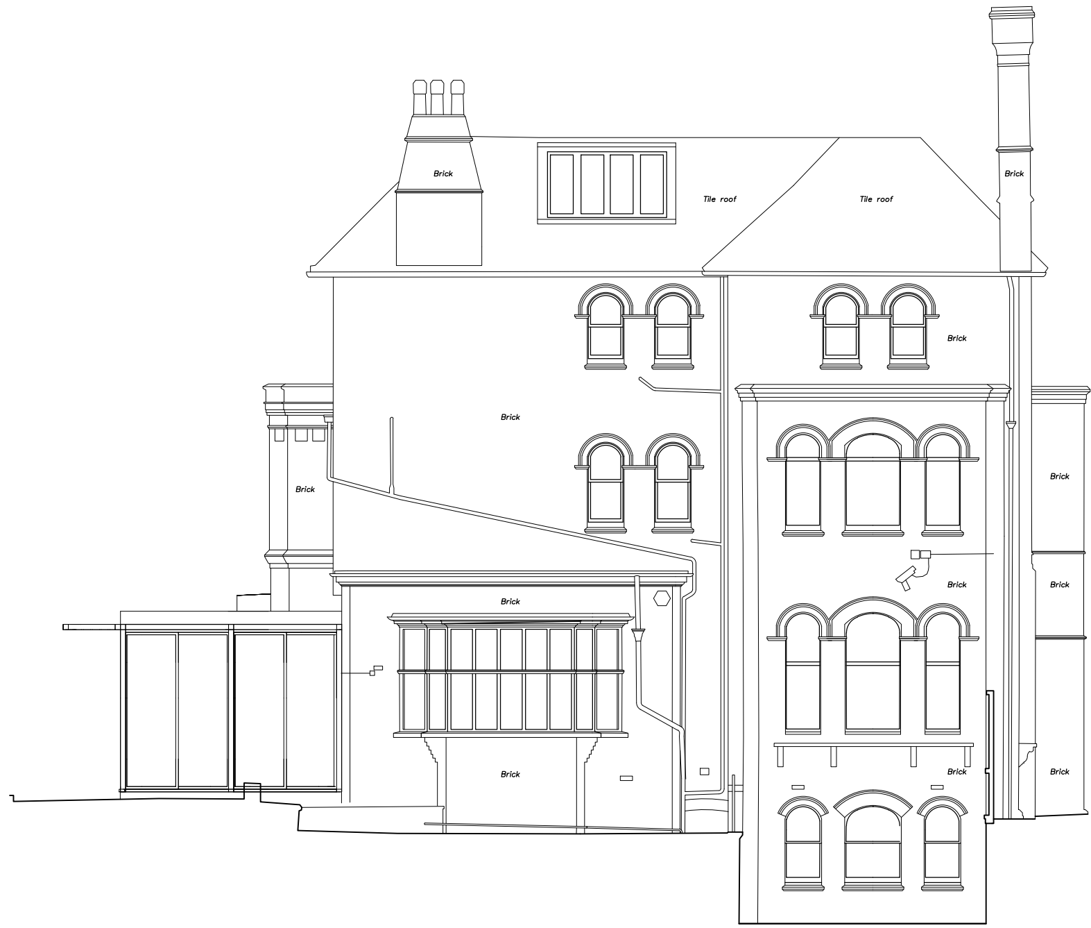
Datum 97.00 Above Site Datum SOUTH SIDE ELEVATION
