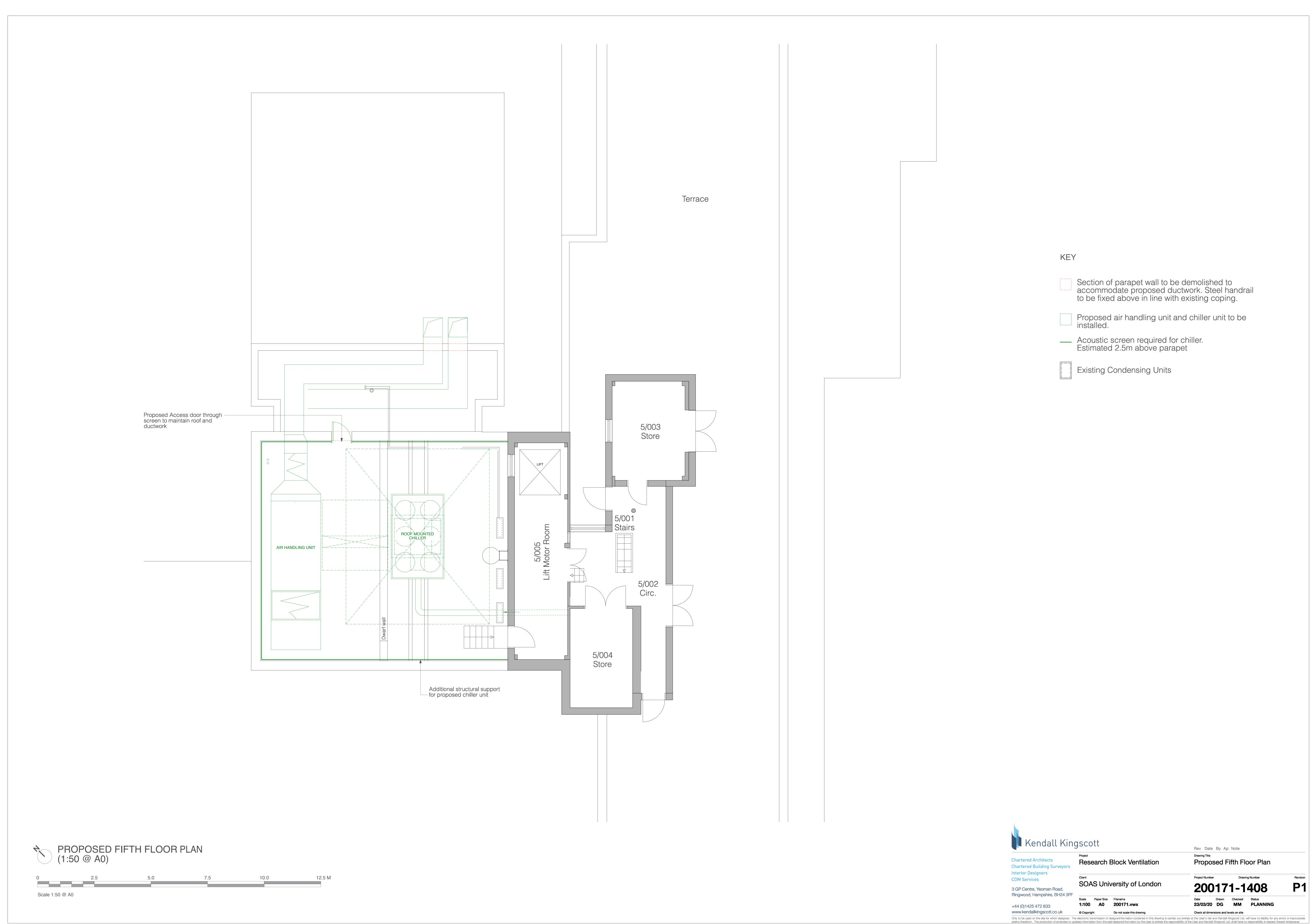
KEY Section of parapet wall to be demolished to accommodate proposed ductwork. Steel handrail to be fixed above in line with existing coping. Proposed air handling unit and chiller unit to be installed. Acoustic screen required for chiller.
