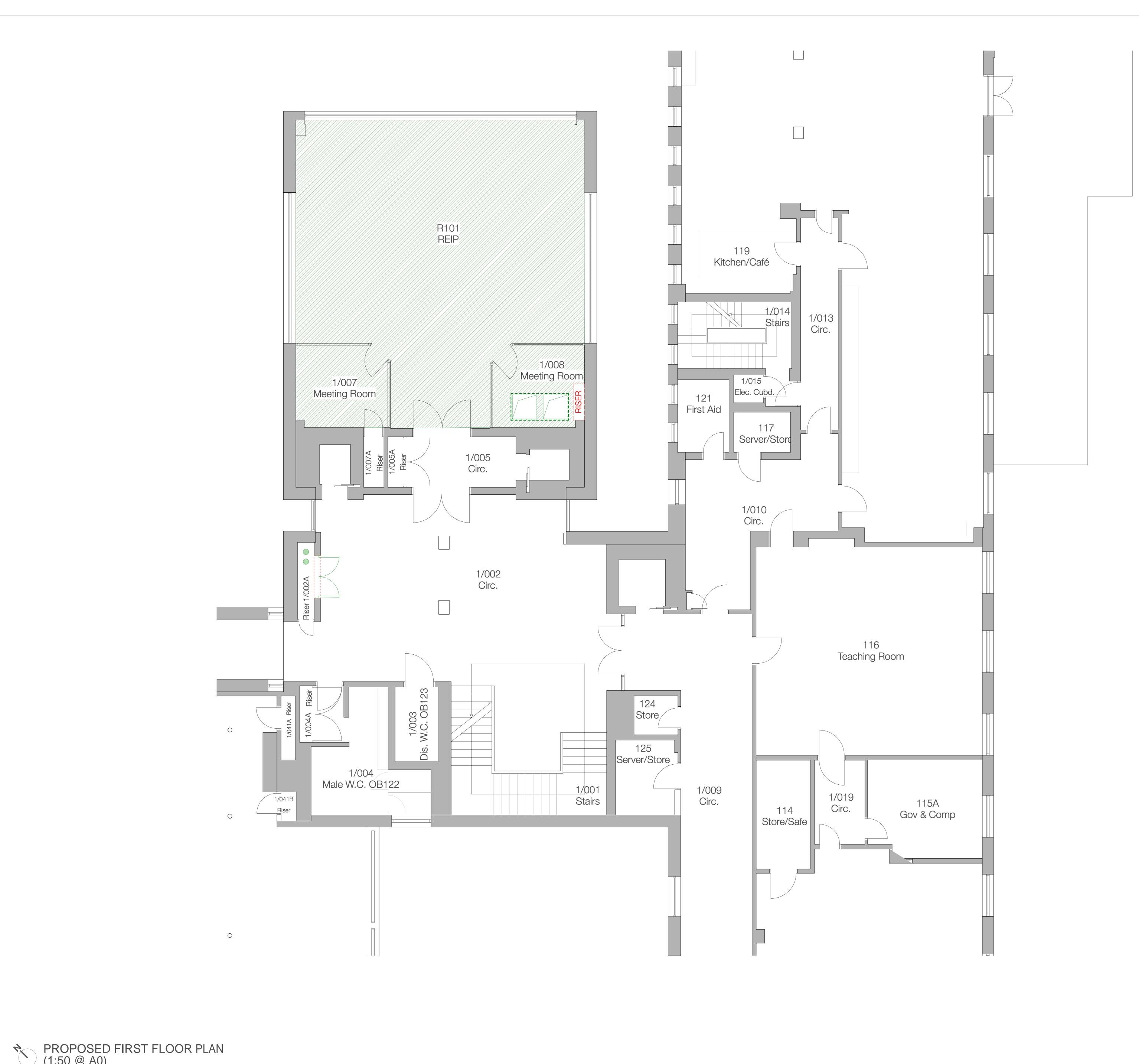
KEY Remove redundant riser and/or vending machine enclosure with associated pipework and power / data Form new double doorset opening for proposed fire rated access doors to riser cupboard Proposed internal pipework route Proposed fresh air and extract ducts Replace existing ceiling and install new fresh air and extract ductwork within ceiling void Proposed plasterboard casing around proposed air ducts
