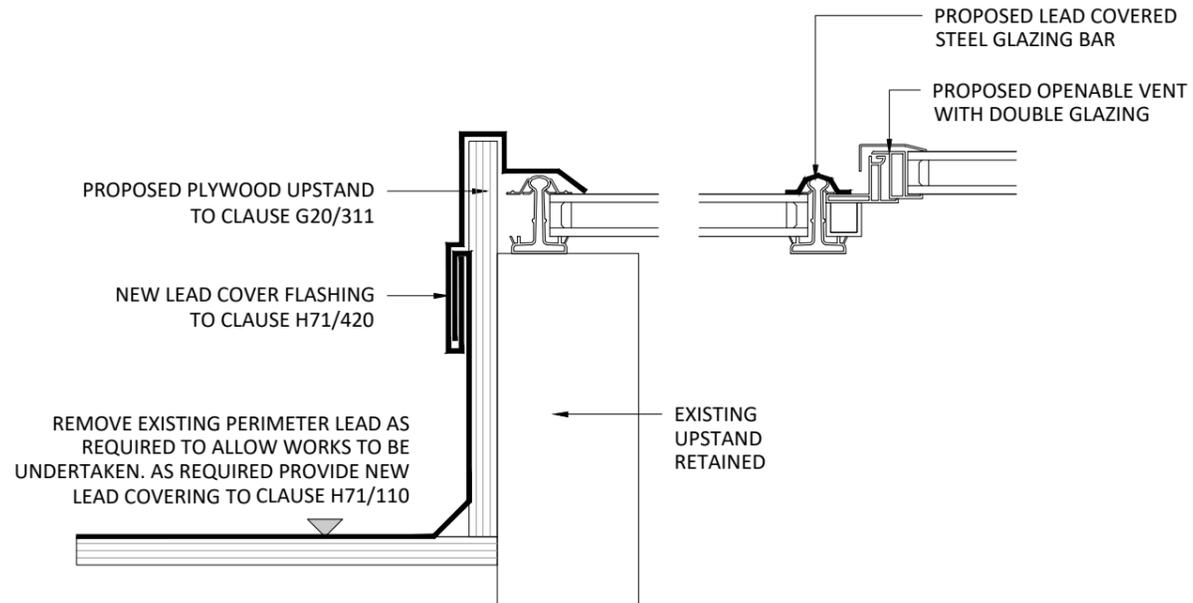
Detail 1 - Typical Rooflight Detail
