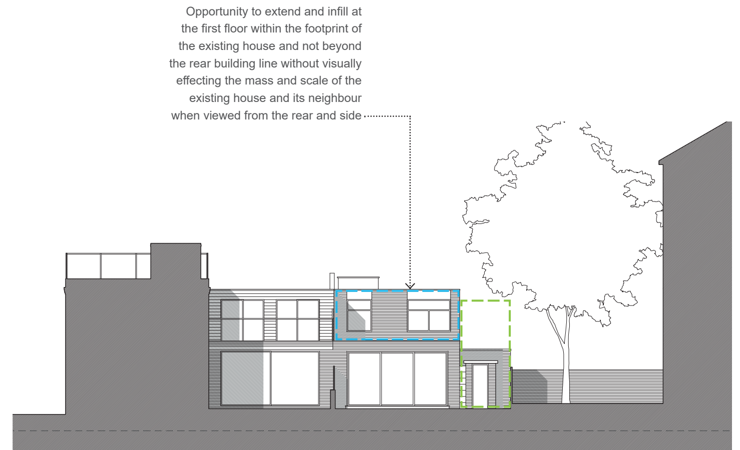
Existing Rear Elevation
