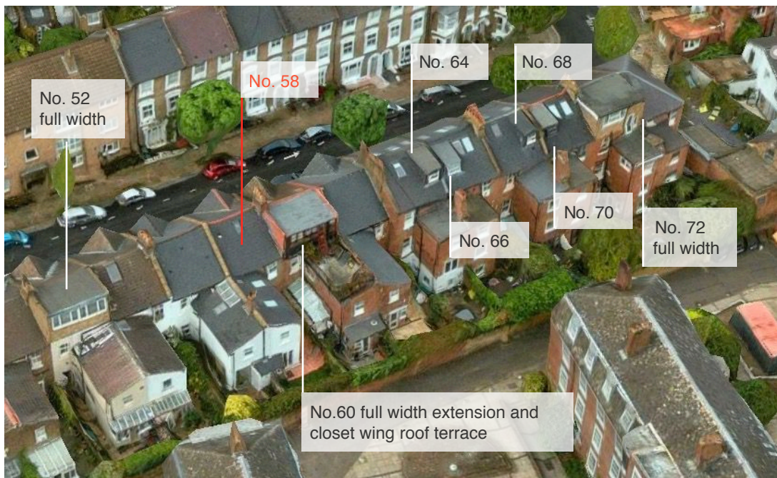
Fig. 02 examples of dormer extension types in the immediate context of no.58 Twisden Road. Note that most dormers – even those with recent planning consents – are unable to maintain Camden’s prescribed 500mm distances from the boundary and the roof ridge, and have been approved in spite of this.
