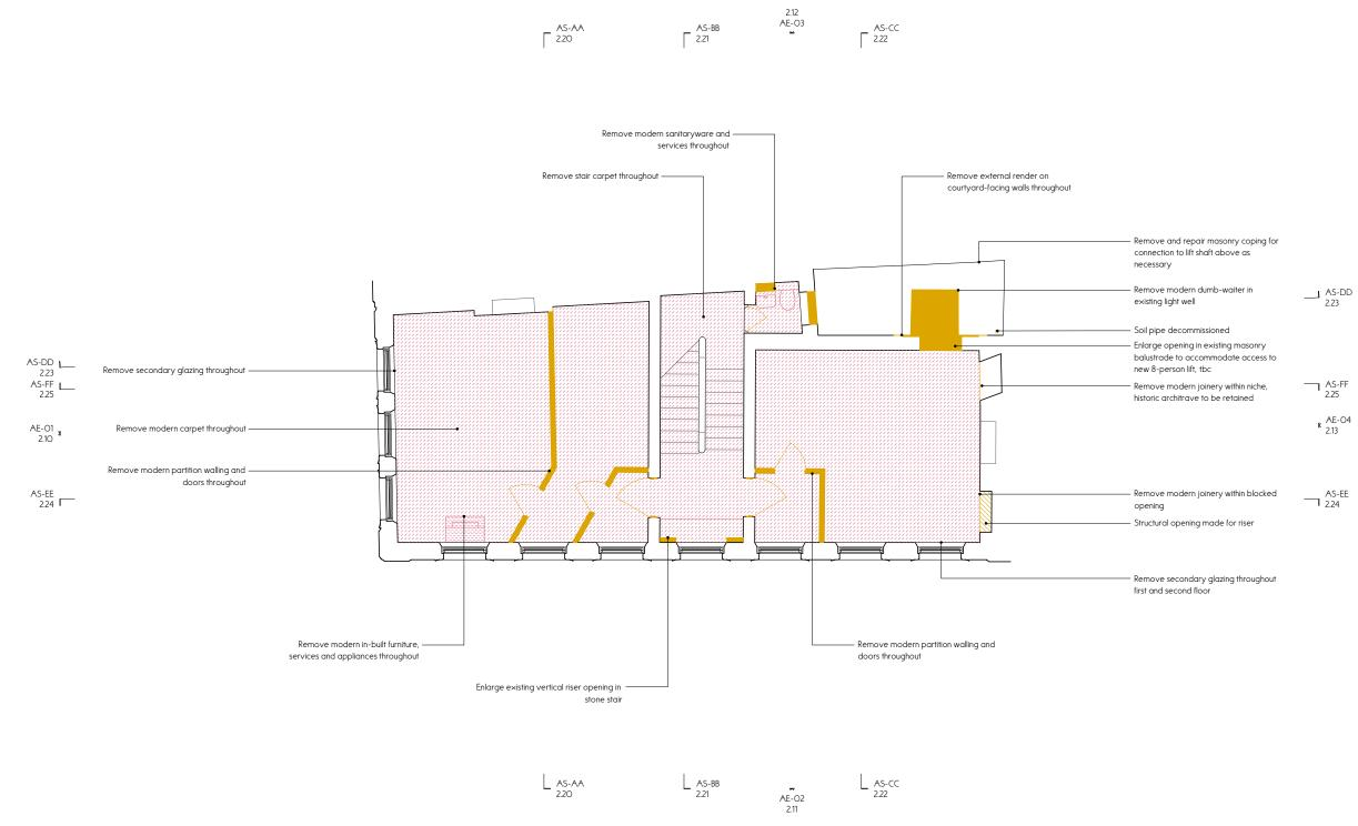
1 DEMOLITION SECOND FLOOR PLAN 2.03 SCALE 1: 100 @ A3
