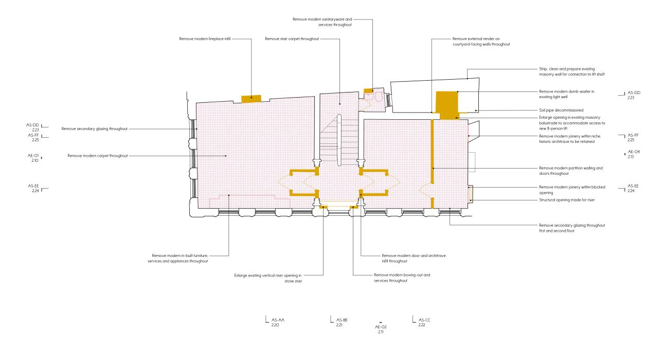
1 DEMOLITION FIRST FLOOR PLAN 2.02 SCALE 1: 100 @ A3
