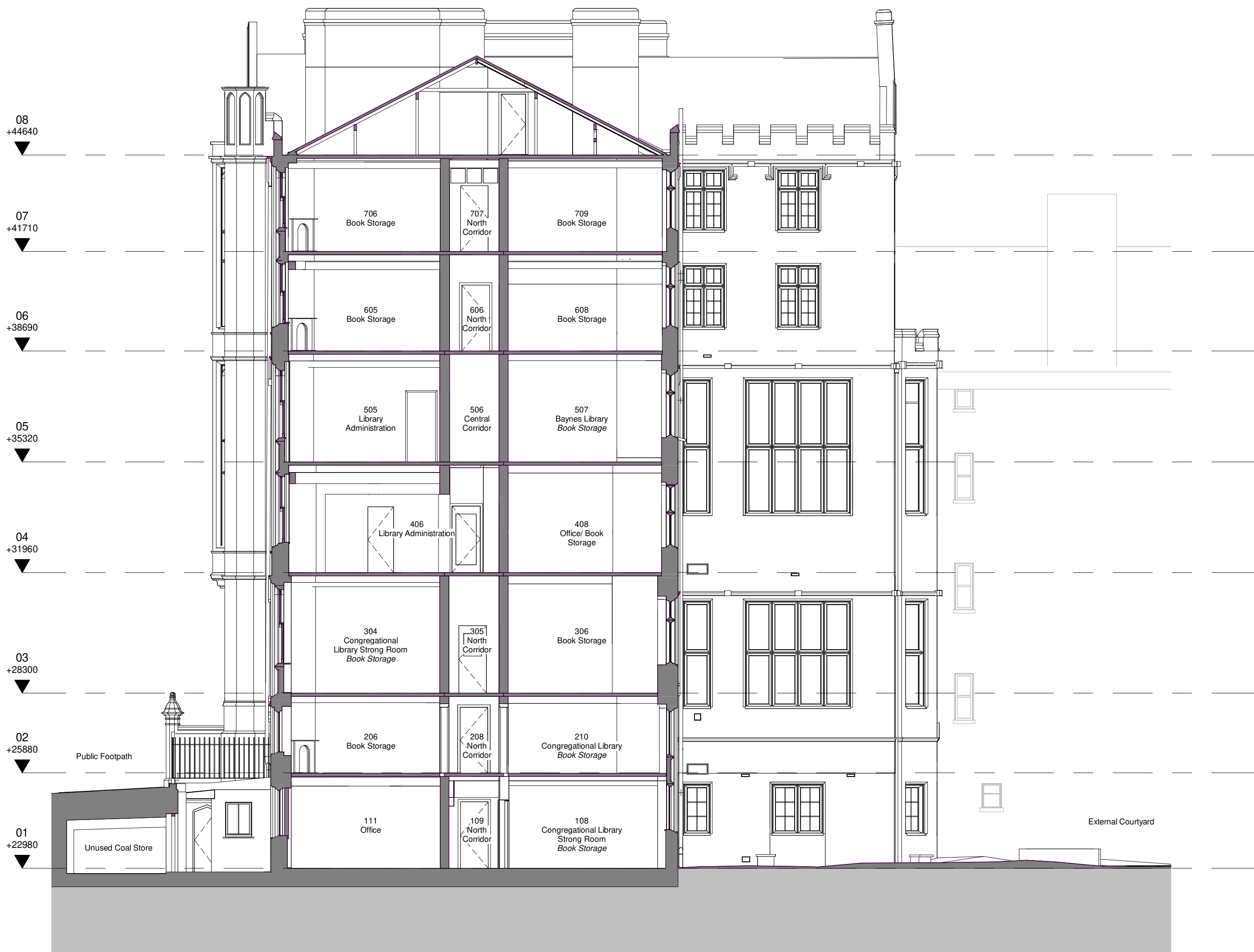
Existing GA Elevation - Central Wing B 1 : 100
