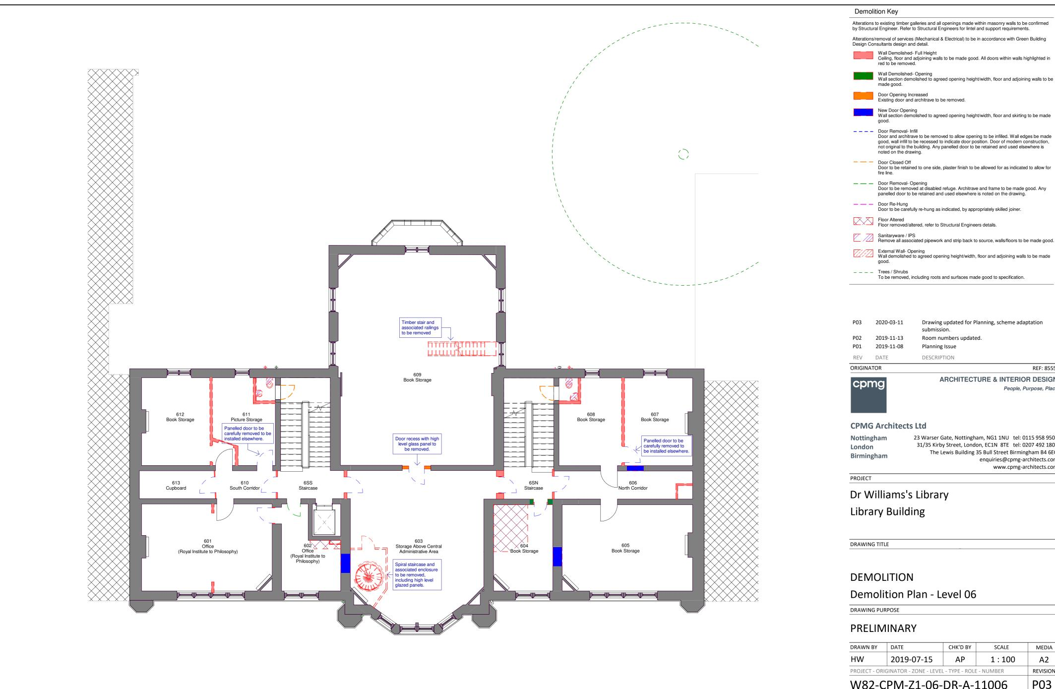
Alterations to existing timber galleries and all openings made within masonry walls to be confirmed by Structural Engineer. Refer to Structural Engineers for lintel and support requirements.
