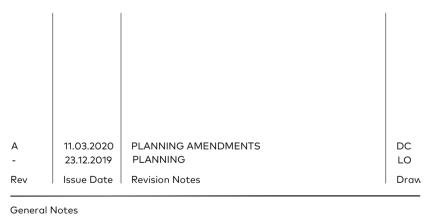
Do not scale. All written dimensions must be checked on site before work commences on site or in shop. Figured dimensions take preference over those scaled. Discrepancies, where identified, must be reported to the Architect immediately. Any areas indicated on this drawing are for guidance purposes only. No responsibility is taken for their accuracy.
