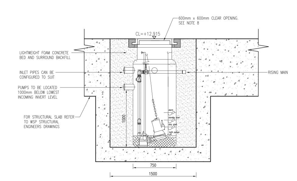
TYPICAL SECTION THROUGH GRP PACKAGE
