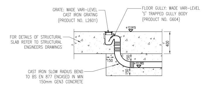
TYPICAL VERTICAL OUTLET TRAPPED GULLY DETAIL BELOW SLAB WITH INVERT LEVEL +12.265
