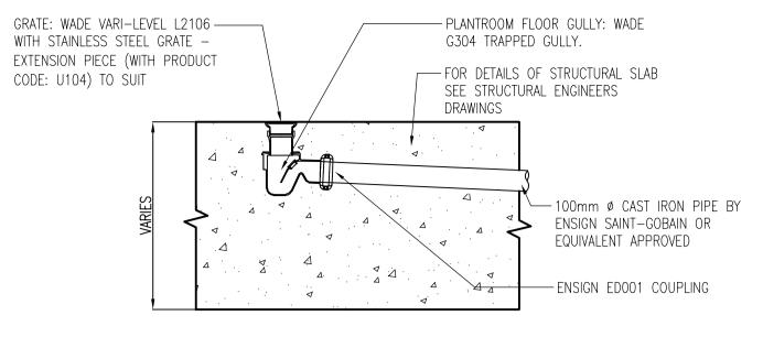
TYPICAL HORIZONTAL OUTLET TRAPPED GULLY DETAIL WITHIN SLAB
