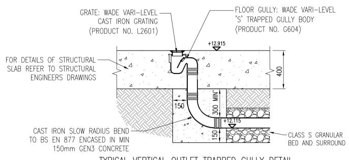
TYPICAL VERTICAL OUTLET TRAPPED GULLY DETAIL
