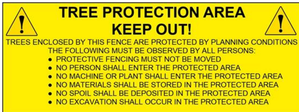
Figure 4. Wording to be included in high visibility all-weather sign attached to protective fencing
