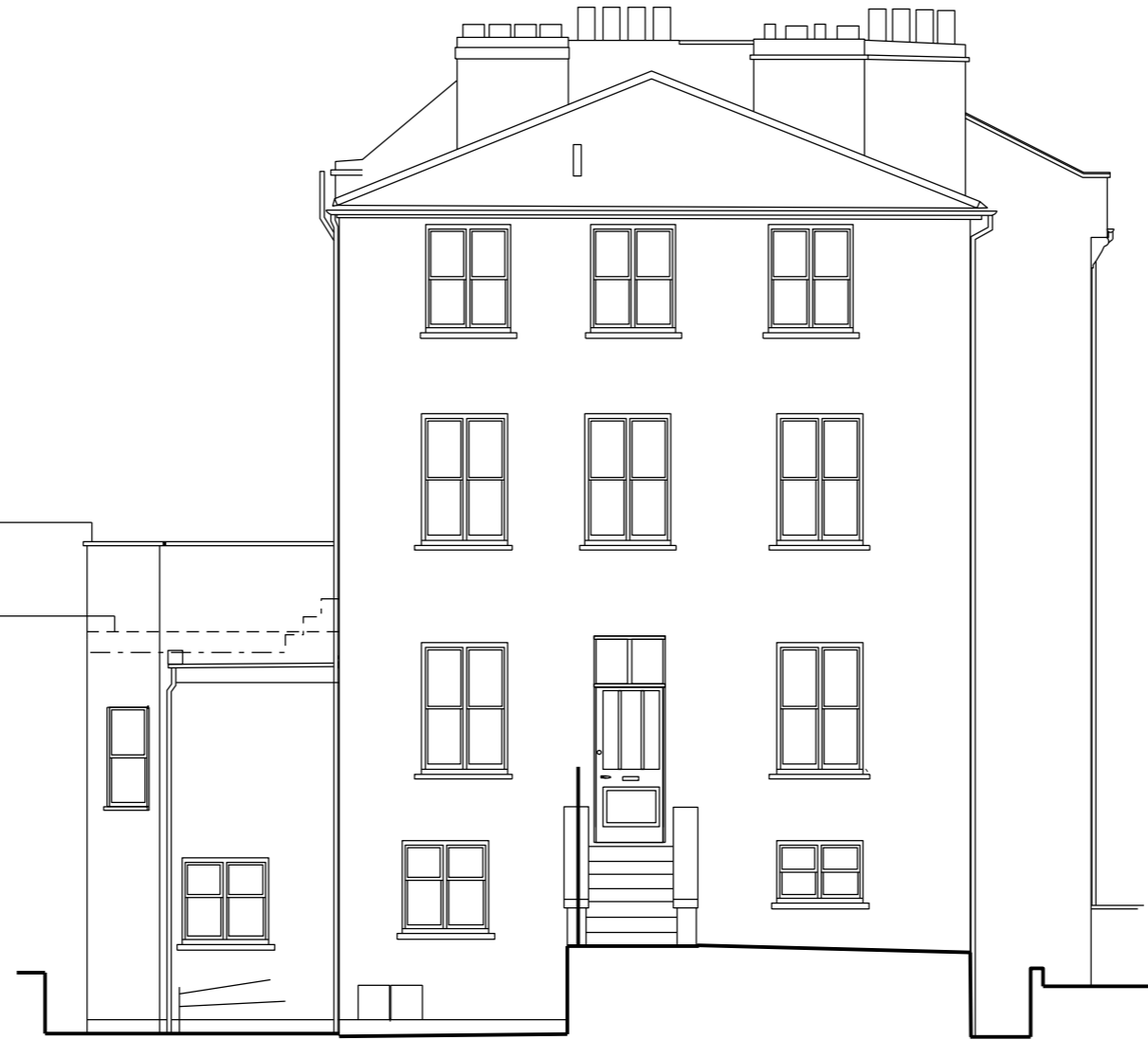
ELEVATION 2 (lower ground and ground floor sash windows and doors replaced to match existing, parapet level raised for balcony)
