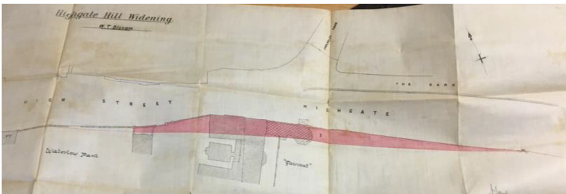
Extent of Fairseat Demolition early 1900s
