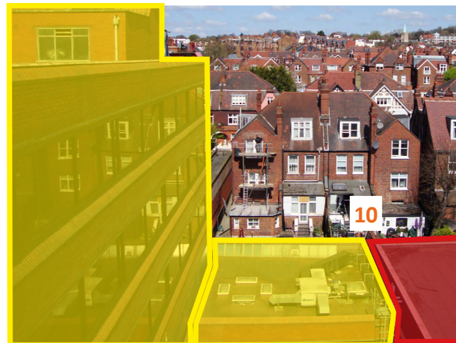
10. Demolish up to external line of one storey building in Phase 2.
