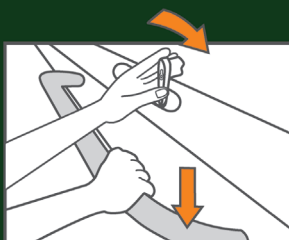
3. Push down on long handle and turn lever. Door will lift automatically.
