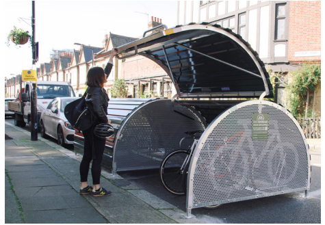
2. Push down on long handle to turn lever Door will lift automatically
