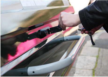
1. Insert and turn key to release lever
