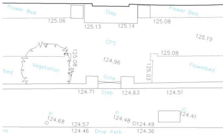
Figure 7: Extract from survey (outline of front of building shown at the top)
