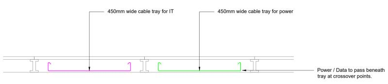
Section B-B - Low Level Electrical Distribution in floor @1:50
