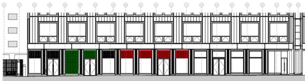
Figure 3: North Building Elevation: Generator Intake (green) & Exhaust (red) Air Louvre Positions
