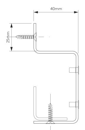
Back panelling to be folded 2mm aluminium stove enamelled satin Black RAL 9005 and to be pre-fitted with M4 riv-nuts for fixing of fascia graphics.
