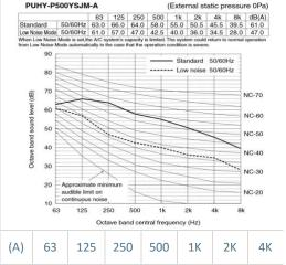
Sound Pressure Level @ 1m from the sides of the AC unit –  $L_{Aeq, 5 \text{ minutes}}$  (dB) Ref 2 x 10<sup>-5</sup> Nm<sup>-2</sup>
