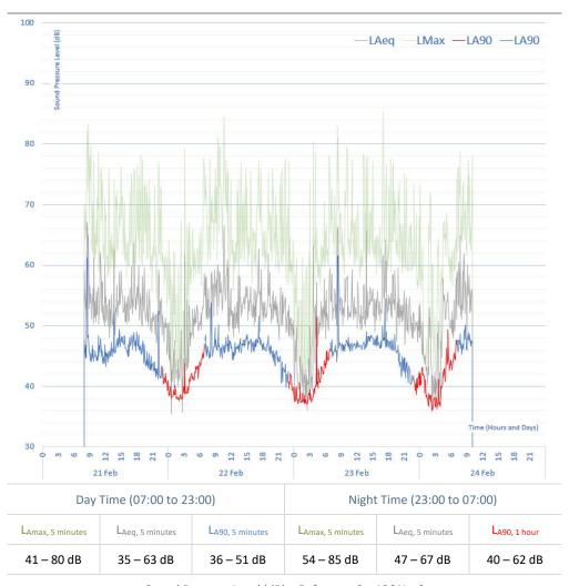
Sound Pressure Level (dB) – Reference 2 x  $10^{-5}\,\text{Nm}^{-2}$
