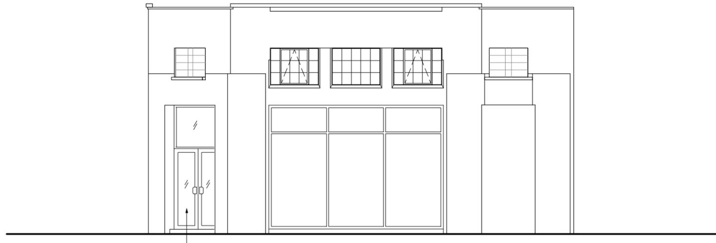
Existing iron framed single glazed entrance door & panel above to be replaced with new powder coated aluminium framed double glazed door & panel - colour and style to match existing
