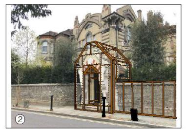
Self supporting timber frame work constructed away from and encompassing all exterior sides and interior faces and continuing along the pavement boundary wall. Padding is to be tightly packed between the timber profile and the supported arch over. Openings for access indicated by white dashed line are shown
