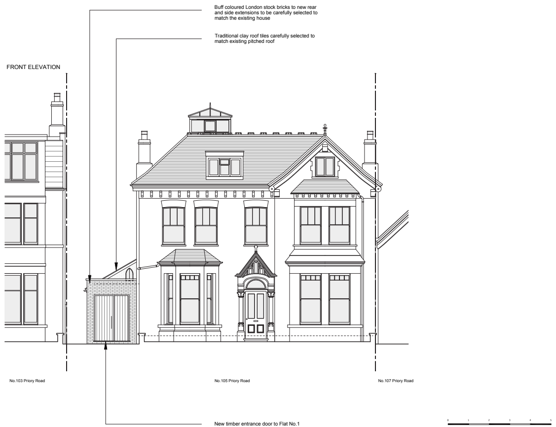
Front elevation drawing showing the proposed new side extension with flat roof and brick parapet to the new front entrance hall and tiled pitched roof to the rear.
