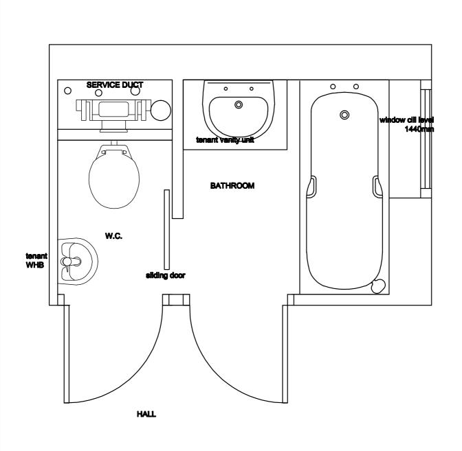
Job: 79J ROWLEY WAY NW8 Title: **EXISTING WC & BATHROOM PLAN LONDON BOROUGH OF CAMDEN** Do not scale from Drawing. All dimensions to be confirmed on all **GRADE II\* LISTED Housing Repairs Service BUILDING** Scale Drawn Job No. Dwg. No. Rev. 0.0 1.0 1:20 |13:09:2019 |6.WILLIAMS| Tel: **020 7874 4444 Pap: 020 7874 557**1
