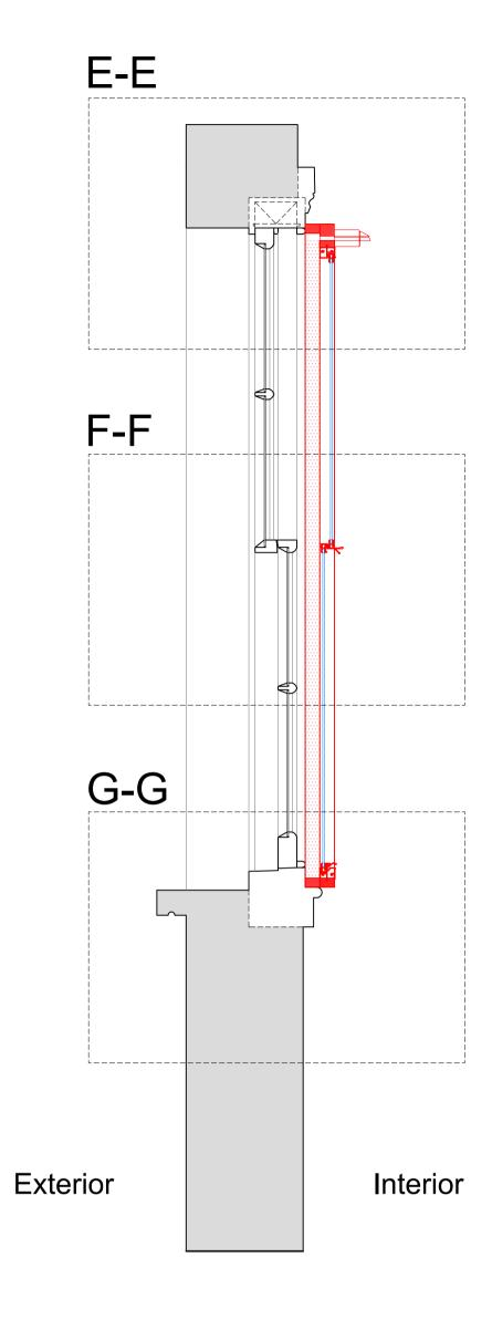
Plan Section B-B with Secondary Glazing Installed
