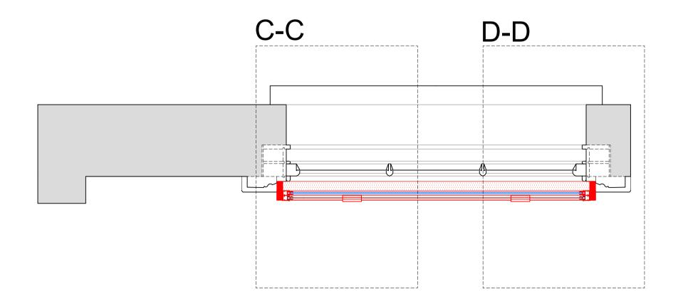
Section A-A through External Wall with Secondary Glazing Installed
