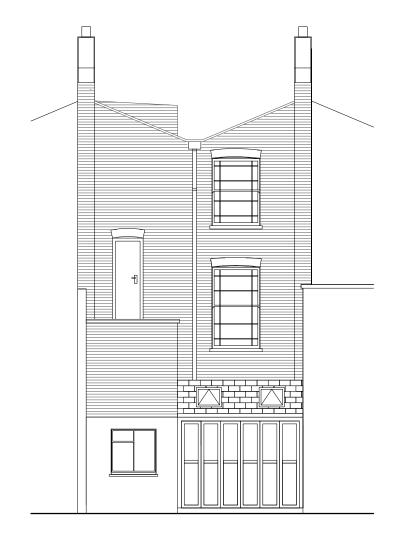
$01 \ \tfrac{PROPOSED \ FRONT \ ELEVATION}{scale \ 1:100}$
