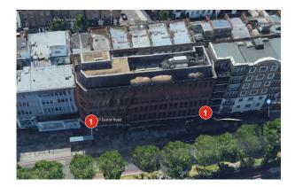
Black powder coated aluminium vertical blade style box signs. Double sided Spaces logo to be fret cut out of both sides with opal acrylic push through letters. Internal LEDs and driver, to illuminate logo on both sides. Fitted to brickwork either end of building.
