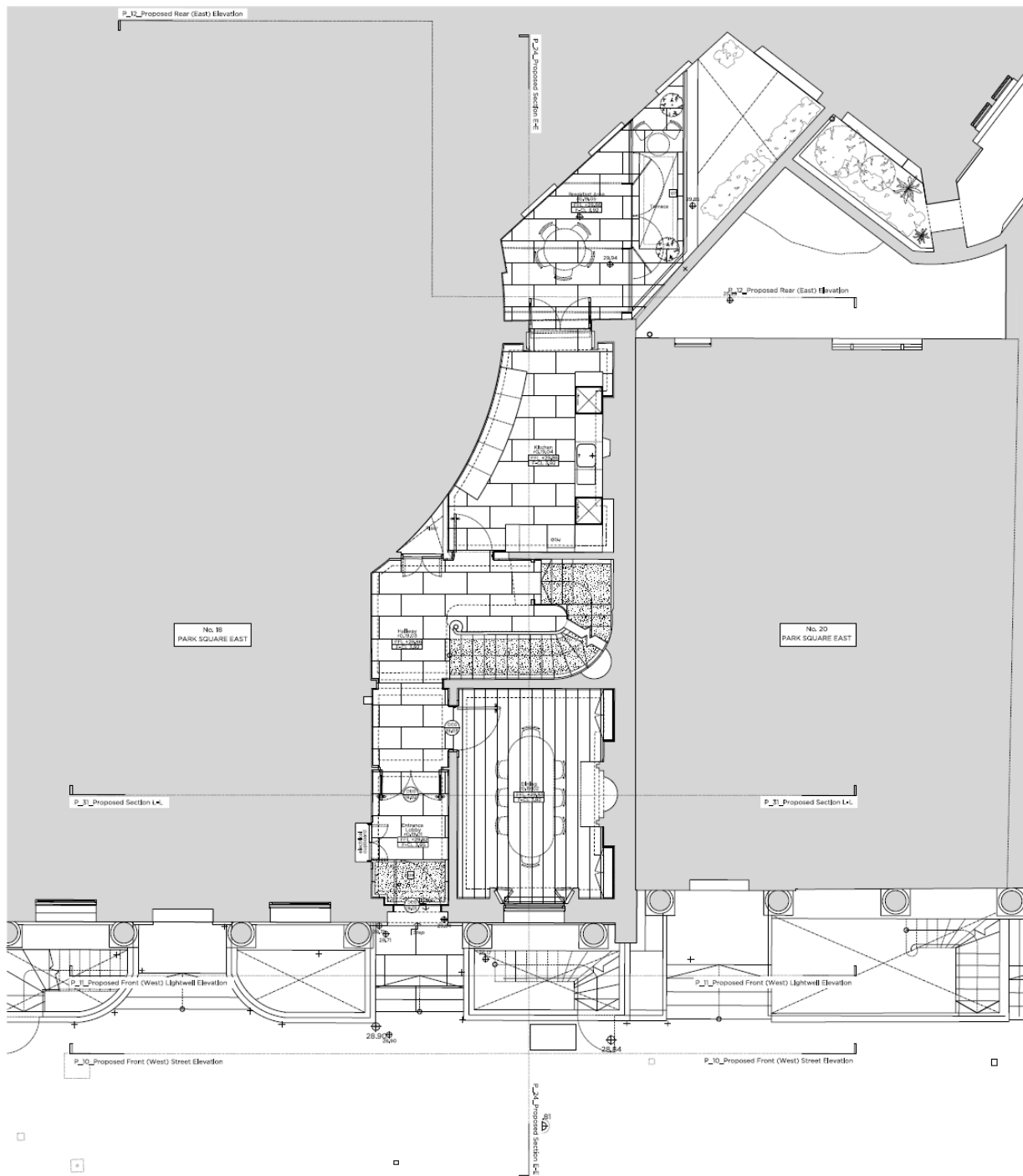
Figure 35 Proposed ground floor plan, showing rear extension. MWA, February 2020.
