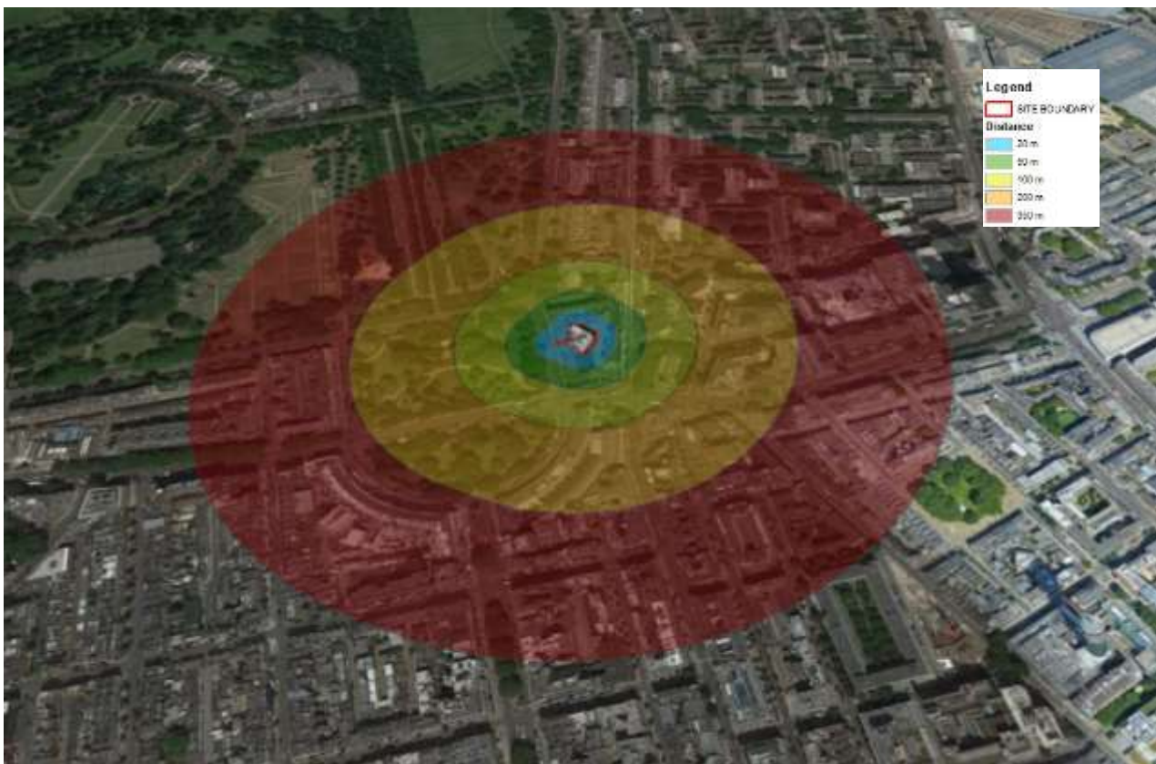
Figure 5 Construction Dust Buffer Zones
