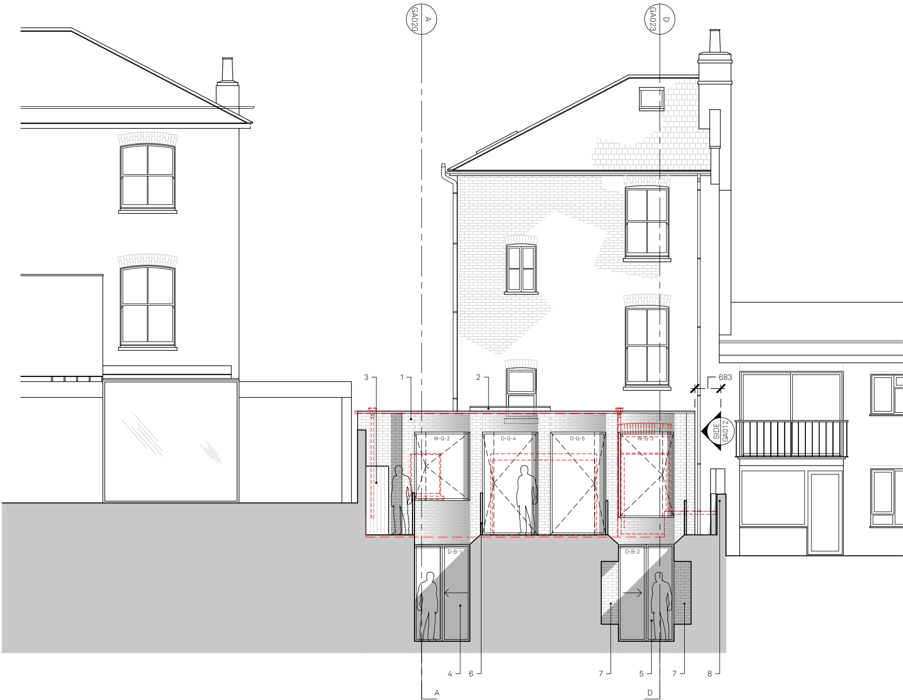
PROPOSED REAR SECTIONAL ELEVATION (WEST) 1:100
