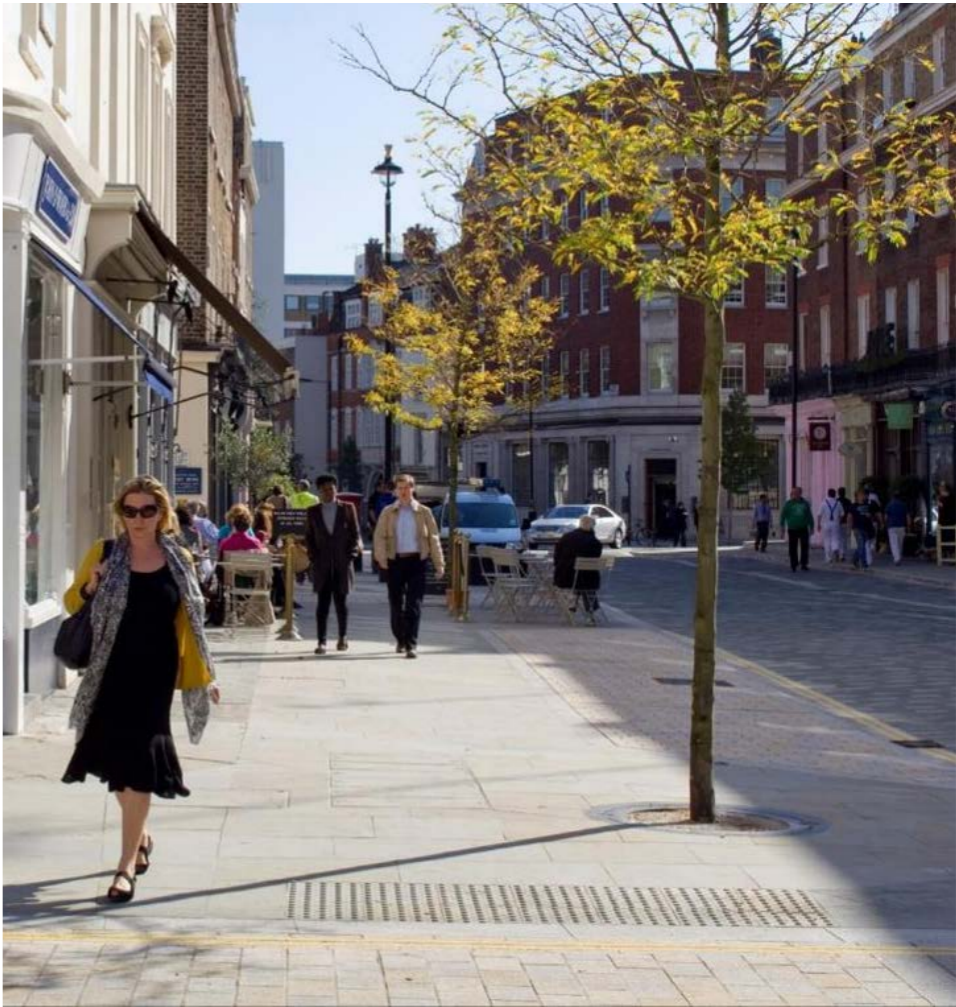
Streetscape Precedent: showing parking pad at street level, tree planting and level setted crossing defined with paving - Buff tri-colour granite setts and English Pennine Stone flag paving
