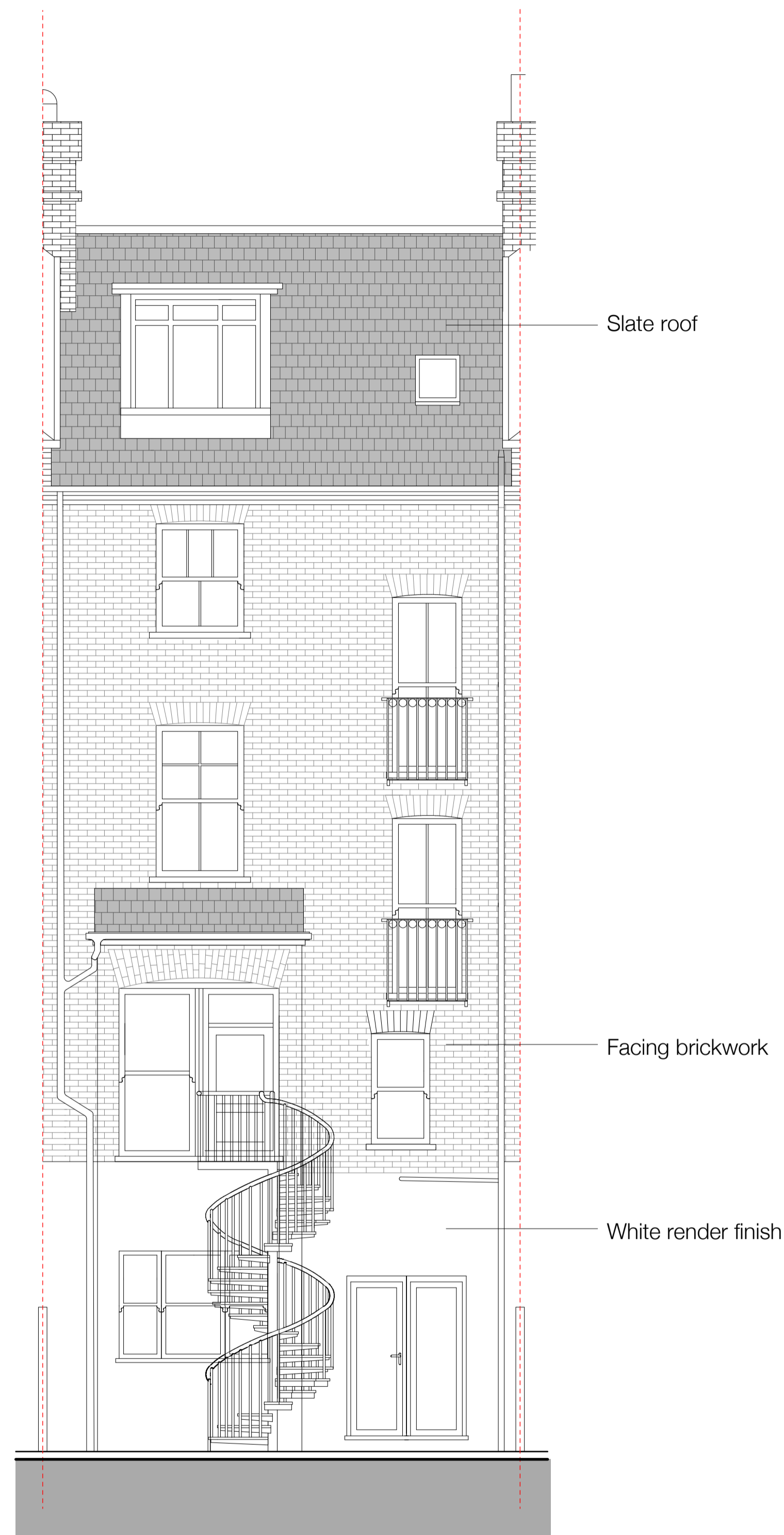
Existing Rear Elevation
