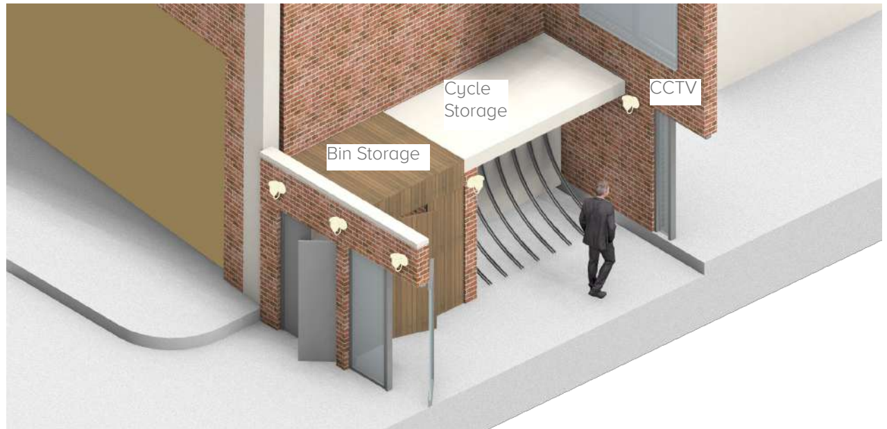
Rear entrance showing Automatic motion sensor wall lamps, Reinforced glazed door, Refuse & recycling storage and cycle storage
