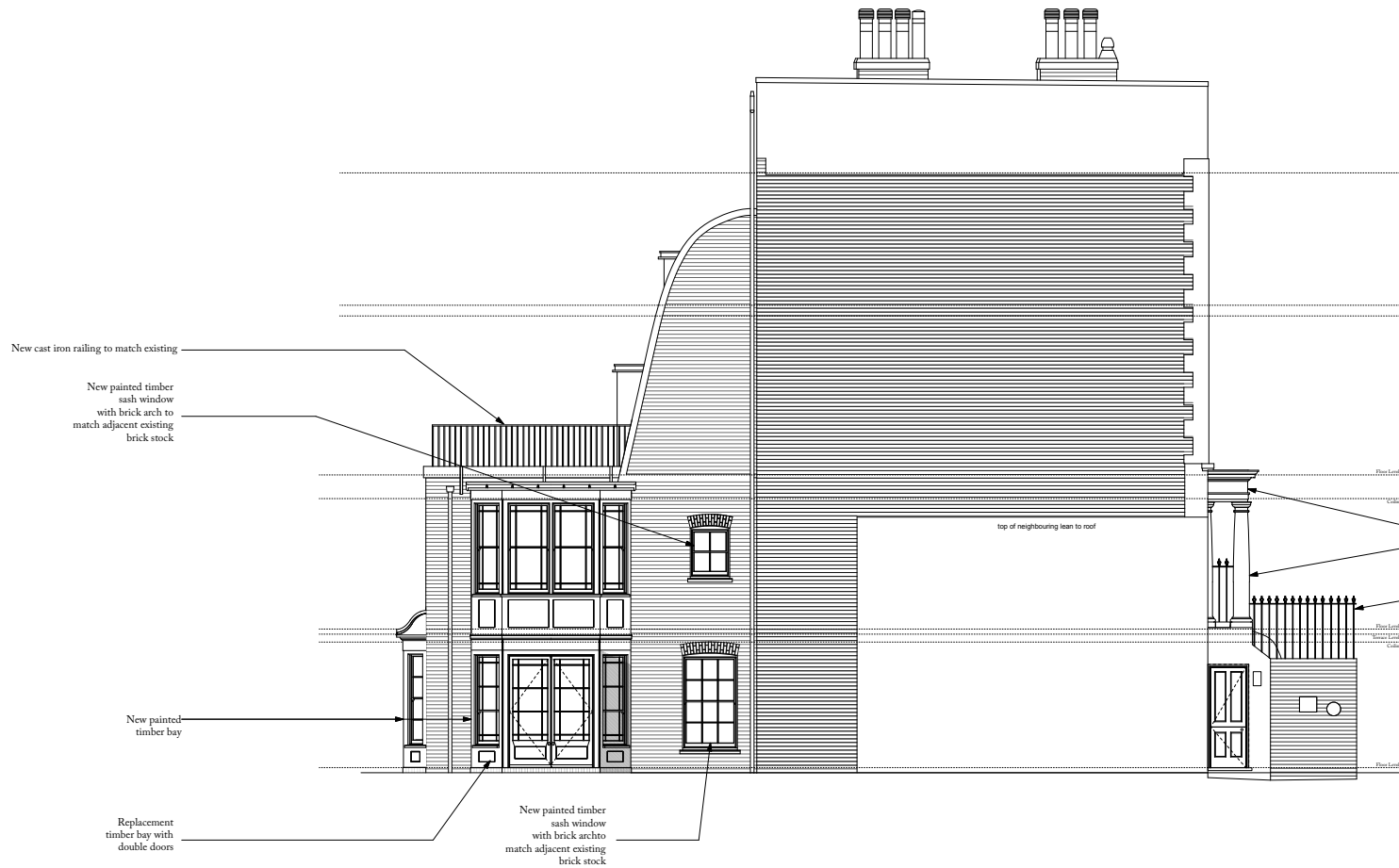
PROPOSED SIDE ELEVATION 1:100 @ A3
