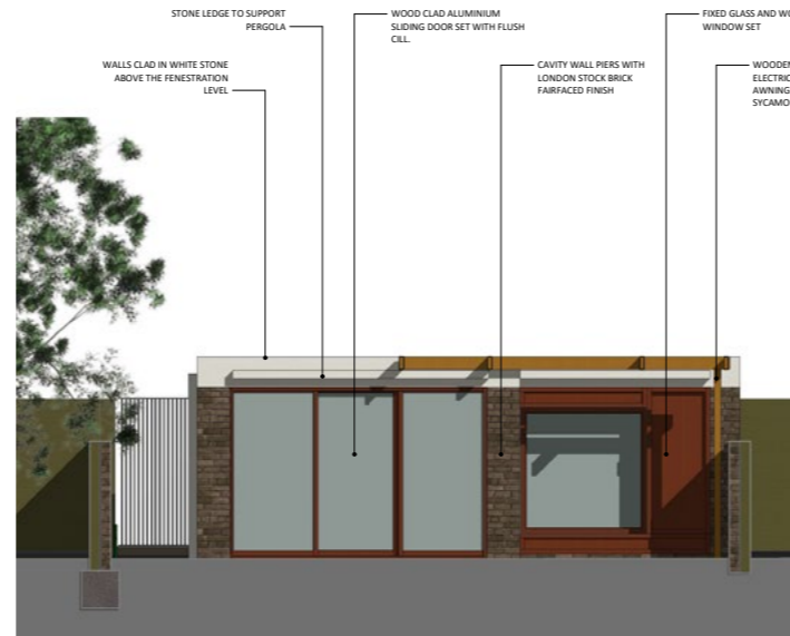
North Elevation of the building
