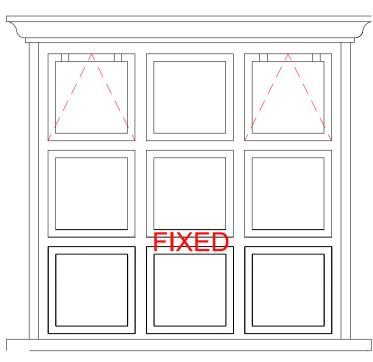
Window No. | W2 No. of Units | 04 Elevation Location | 1, 2 Glass Type | Single Glazing
