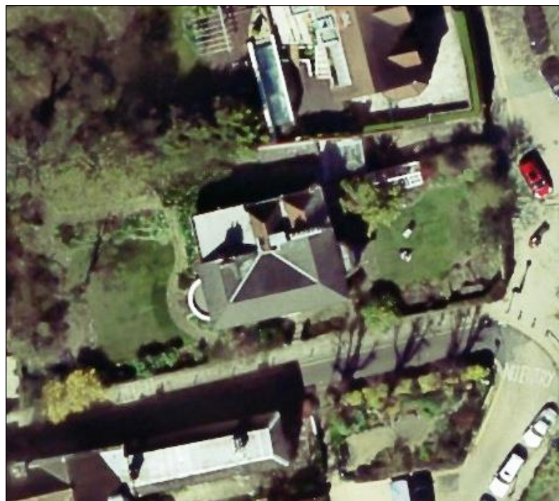
Plate 14 - Aerial photograph of current roof of Vine House showing loss of central gully and two pitches to the rear (Getmapping 2015)
