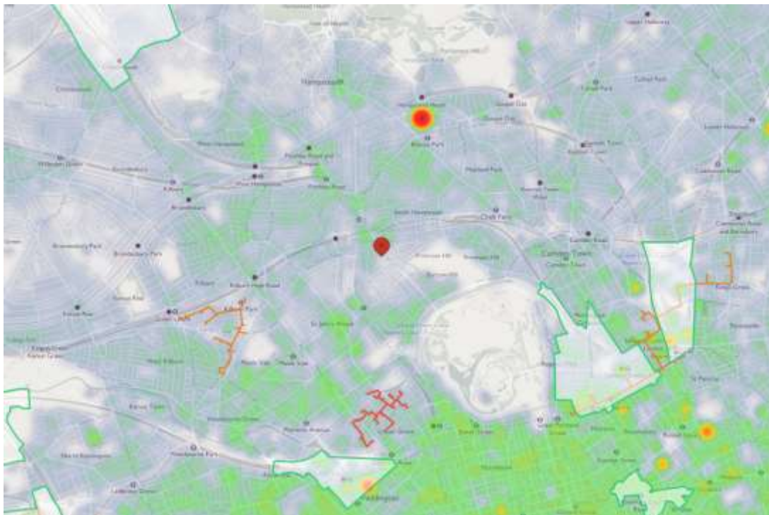
Figure B2: London Heat Map tool showing existing heat networks in red line, proposed heat networks in orange and Opportunity Area Planning Framework zones outlined in green
