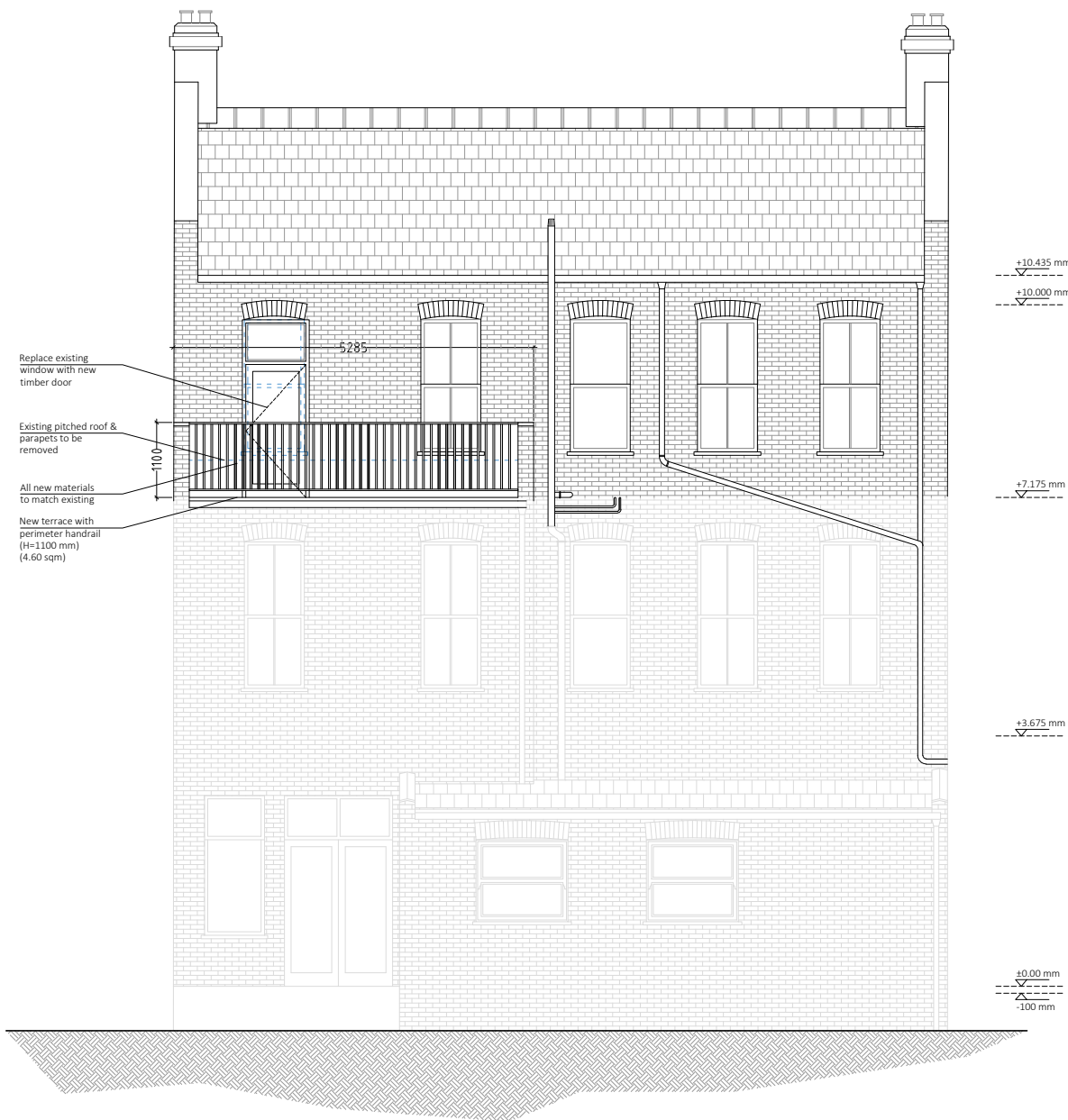
EXISTING REAR ELEVATION
