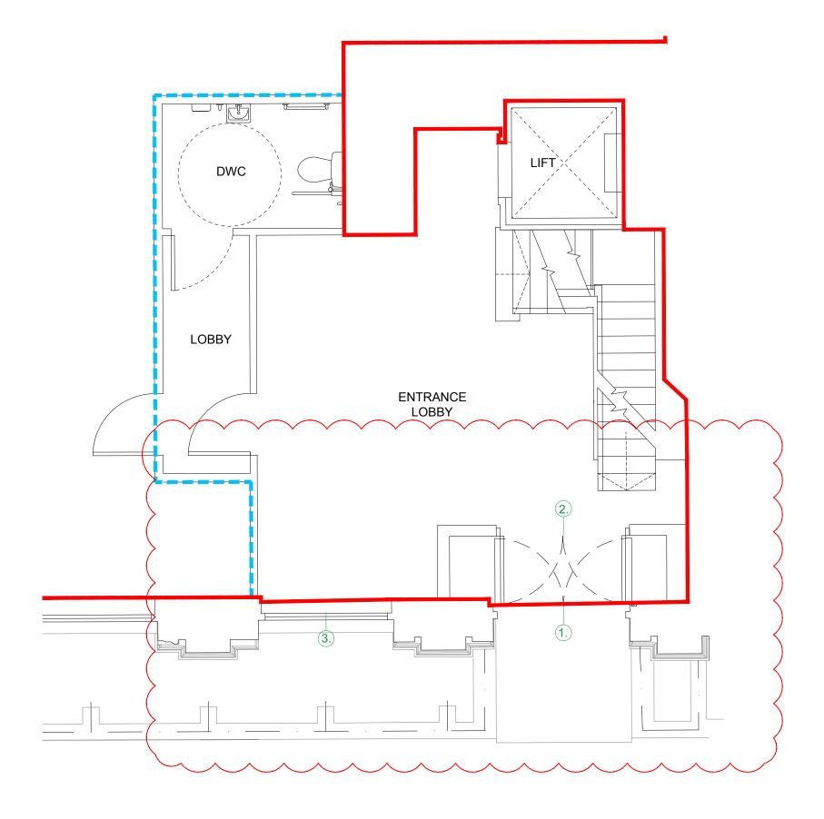
date 17.12.19 Entrance door position retained, platform lift omitted, windows amended, railings retained
