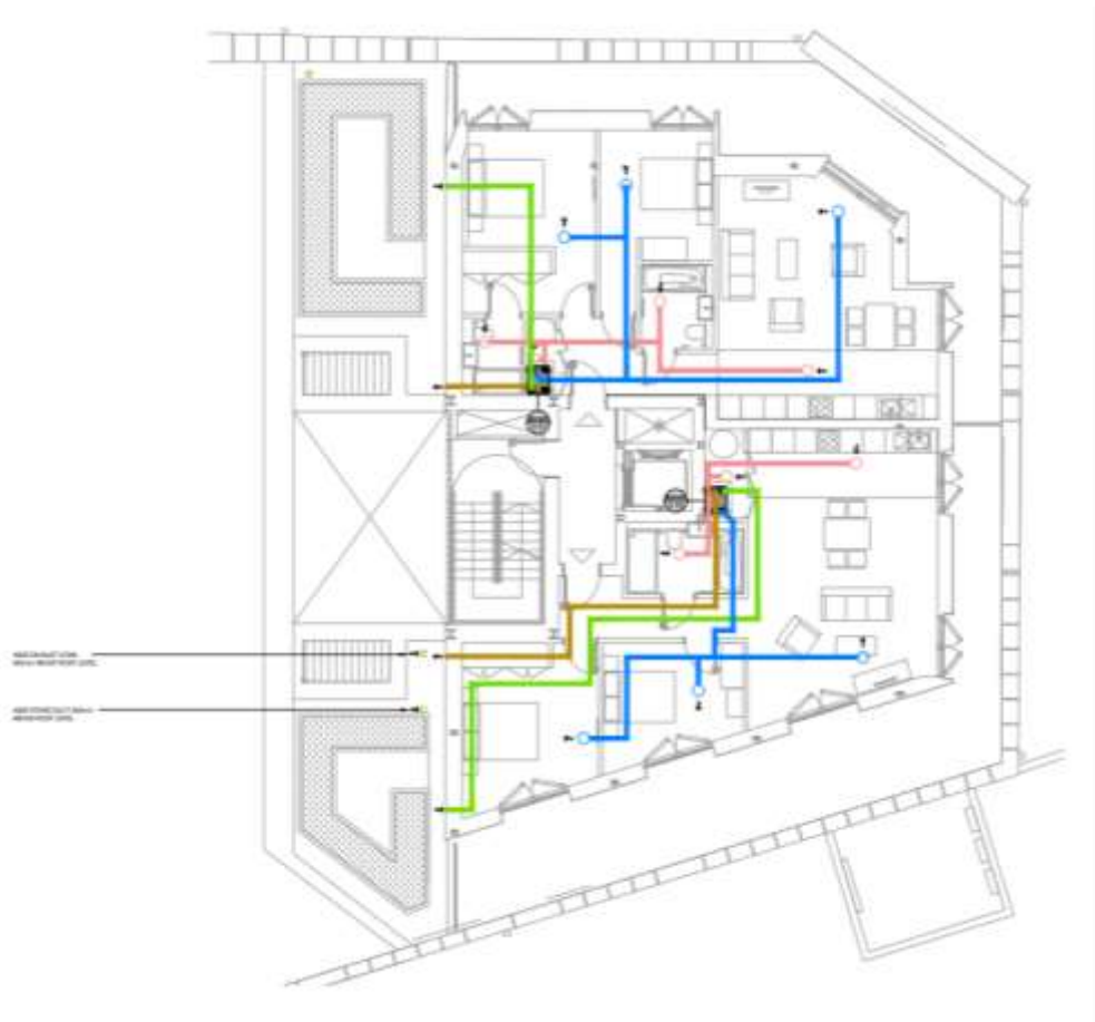
Figure 4: Residential units– Floor 3 (units 3.1 to 3.2) showing proposed mechanical ventilation with heat recovery
