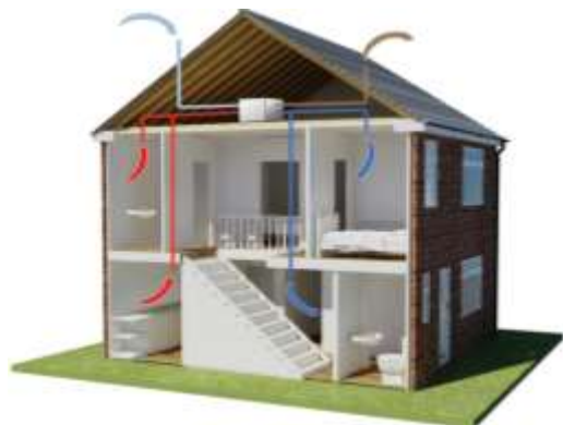
Figure 7: Typical domestic MVHR system.
