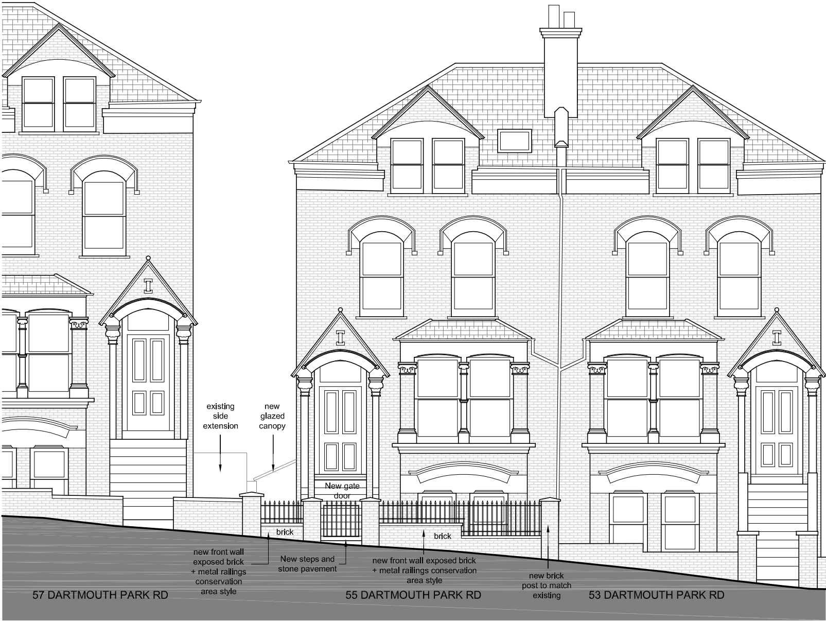
PROPOSED - Front Elevation Scale 1:100@A3 PA-04
