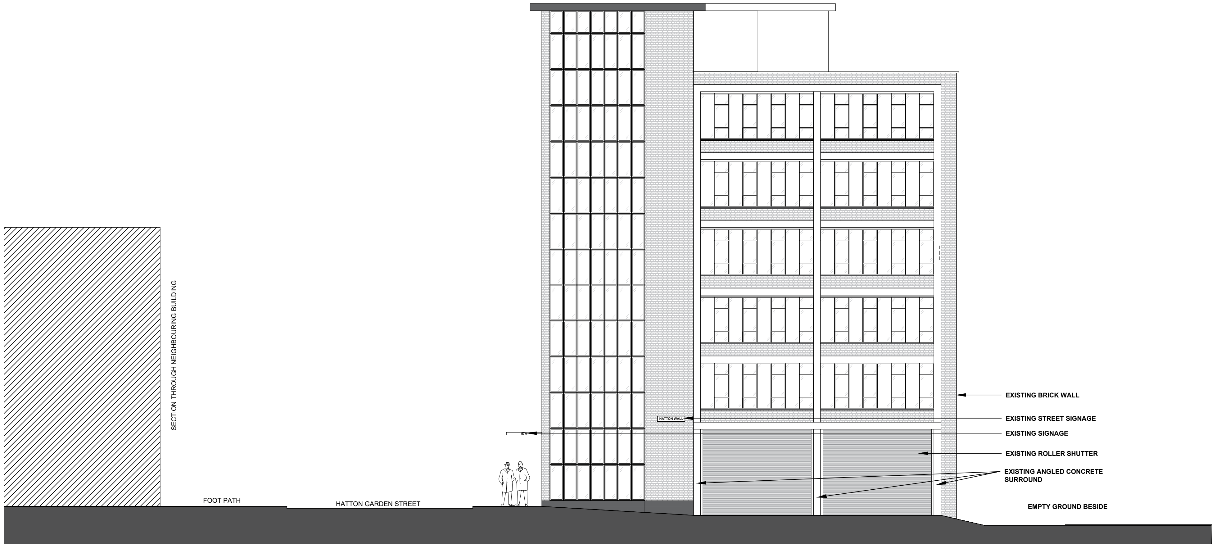
EXISTING S/E ELEVATION - HATTON WALL SCALE 1:100
