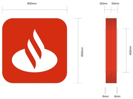
Folded aluminium projecting sign powder coated RAL3020 with fret cut push through 050 acrylic logo Size - 600mm x 600mm x 100mm Logo height - 400mm Internally illuminated to logo only via LED Illumination does not exceed 250 candelas per meter square
