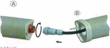
Plug Male & Female Connector Together & Twist to Seal
