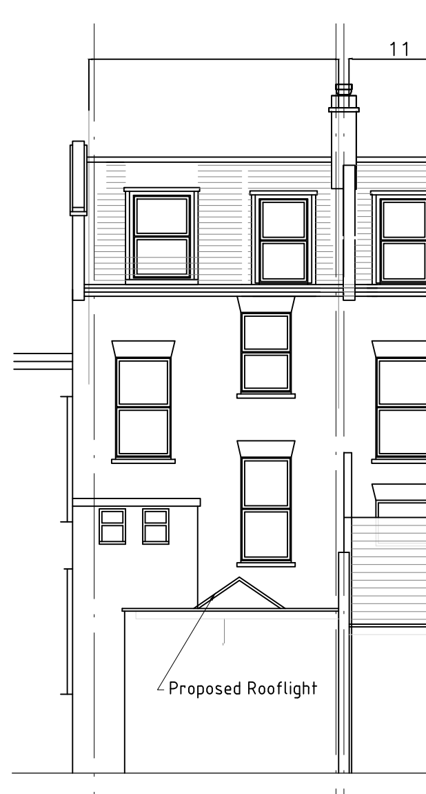
REAR ELEVATION AS PROPOSED SCALE 1:100 @A1
