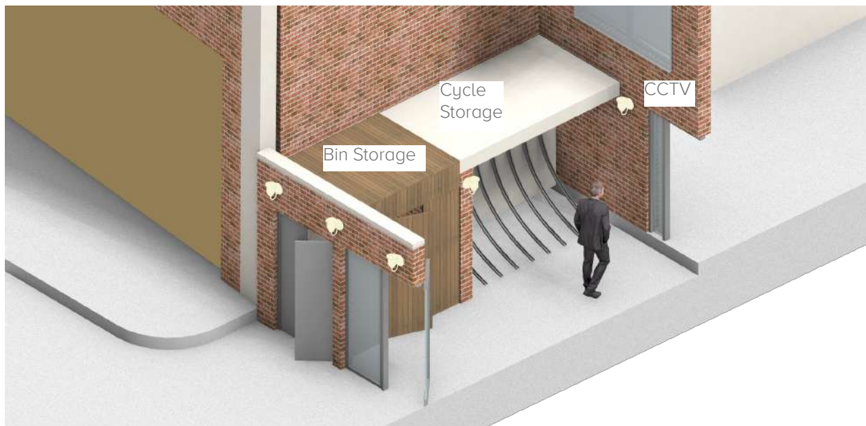
Rear entrance showing Automatic motion sensor wall lamps, Reinforced glazed door, Refuse & recycling storage and cycle storage
